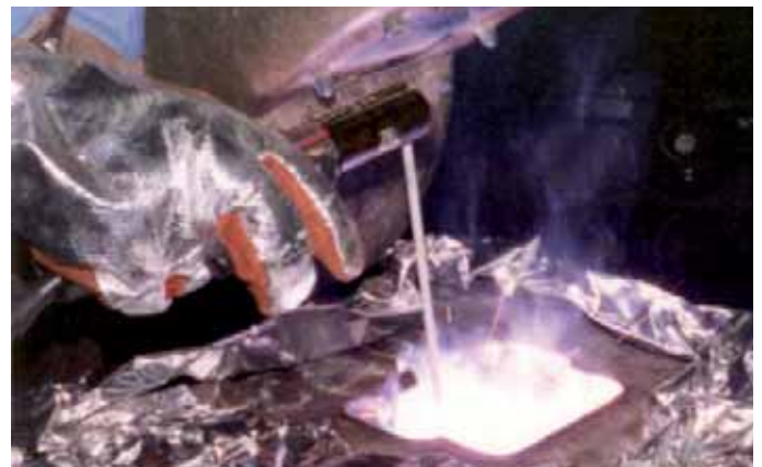
Manual arc welding and covering of components
