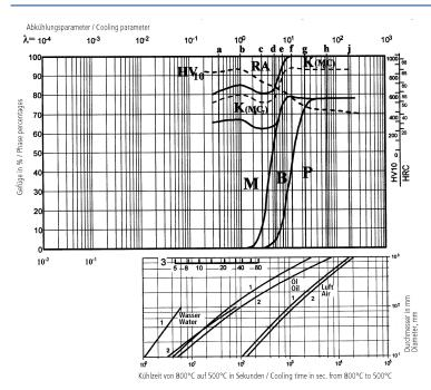
A....Austenite B....Bainite K....Carbide P....Perlite M....Martensite RA...Retained Austenite
