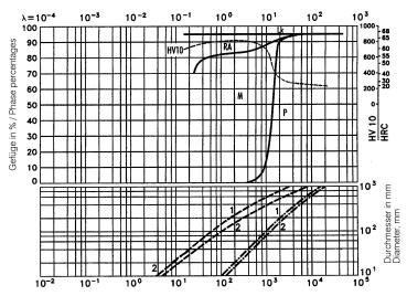
HV10... Vickers Hardness LK... Ledeburitic carbides RA... Retained austenite M... Martensite P... Perlite
