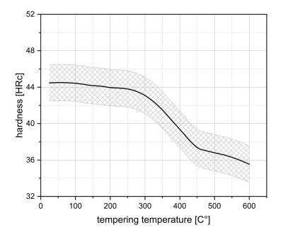
**Heat treatment** Hardening temperature 850°C Soaking time 30 min water quenched
