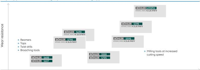
Property profile of BÖHLER high speed steel for cutting applications
