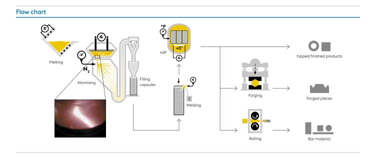
High purity, homogeneous alloyed powders, with appropriate particle size and distribution are subjected to a high pressure, high temperature process to obtain a homogeneous, segregation-free tool steel withvirtually isotropic properties.
