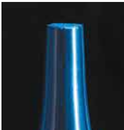
Brittle material (brittle fracture)
